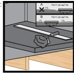
Floor pavement positioning with a 1% gradient. Installation variation A: ONE SIDED GRADIENT.
