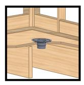
Screw the Drain Base Flange of the drain into the hole with 4 wood screws. The top surface of the drain base should be flush with the top of the wood floor.
