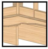
Cut a tapered hole into the floor. Make sure the area under the floor is clear for plumbing. Notice 2x6 boards between studs will surround the shower walls.
