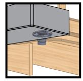
Depending if you are going to use the rubber gasket or adjustable ring, you will either thread in the adjustable version or put in the rubber coupling. Shown above is the adjustable ring. They are not meant to be used together. One or the other.
