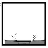
The floor cover must be placed accurately and attached to the material.
