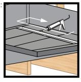
The floor and shower drain must be filled with adhesive.
