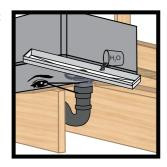
Align with the level of shower drain and connect the siphon with adapter to the outlet.
