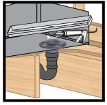
Before the shower drain is installed on the flange, use a silicone ring to fix and then install it into the flange.
