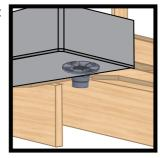
Place the clamping ring over the flange tighten with bolts. This will push the rubber liner in the center downward where you cut the "X".
