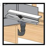
Before the installation of the shower drain, construction protection materials (such as polystyrene piece, available in the package) should be placed.
