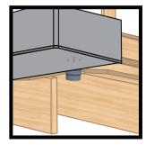
Using a sharp utility knife, cut a small slice into the rubber above the 4 holes where the 4 bolts will thread into. Push the bolts thru each slice and thread into drain base a few turns. In the center of the drain, slice an "X" into the rubber, no wider than about 2 inches.
