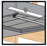
Remove the protective material and clean the residue at the bottom.
